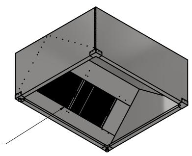
Stainless Steel-Baffle Filters (Included)
