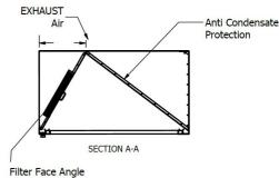
Filter Face Angle 30 Deg as required by AS1668
